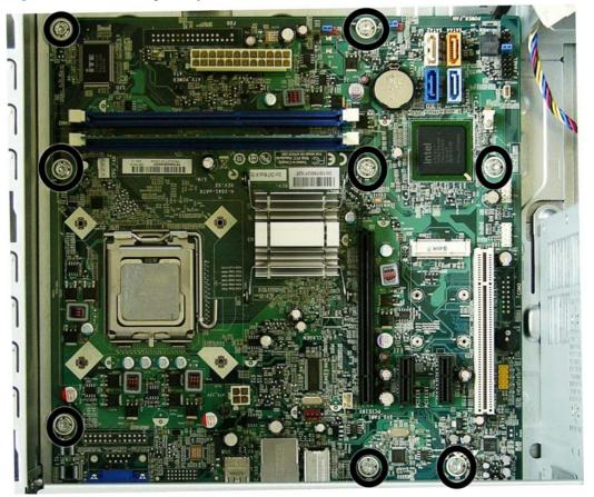
Figure 2-60 Removing the system board — model 500B shown
